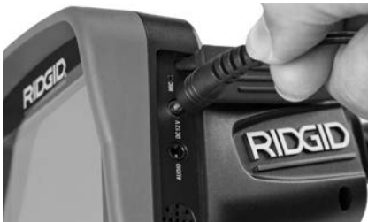
Figure 6 – Powering the Unit with AC Adapter
